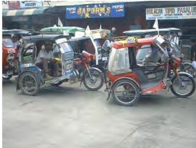
*Tricycles are motorcycles attached to or covered within a steel cab. These are common and inexpensive transports typically for distances of a few kilometers.*
